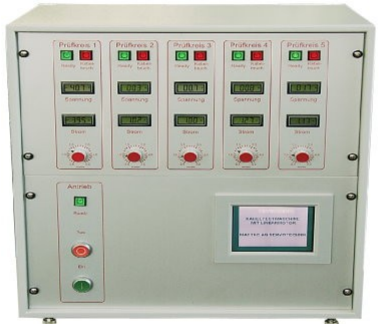
Control system for 5 cables
