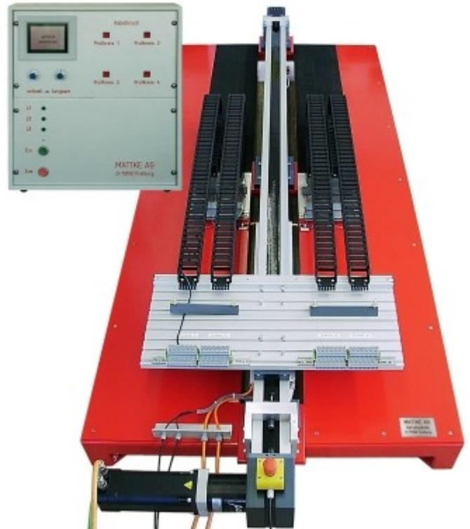
Test table with control panel.
