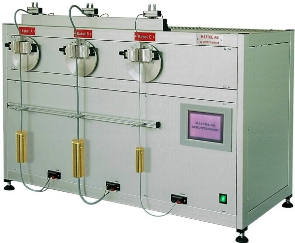
3-axis Cable bend-test machine
