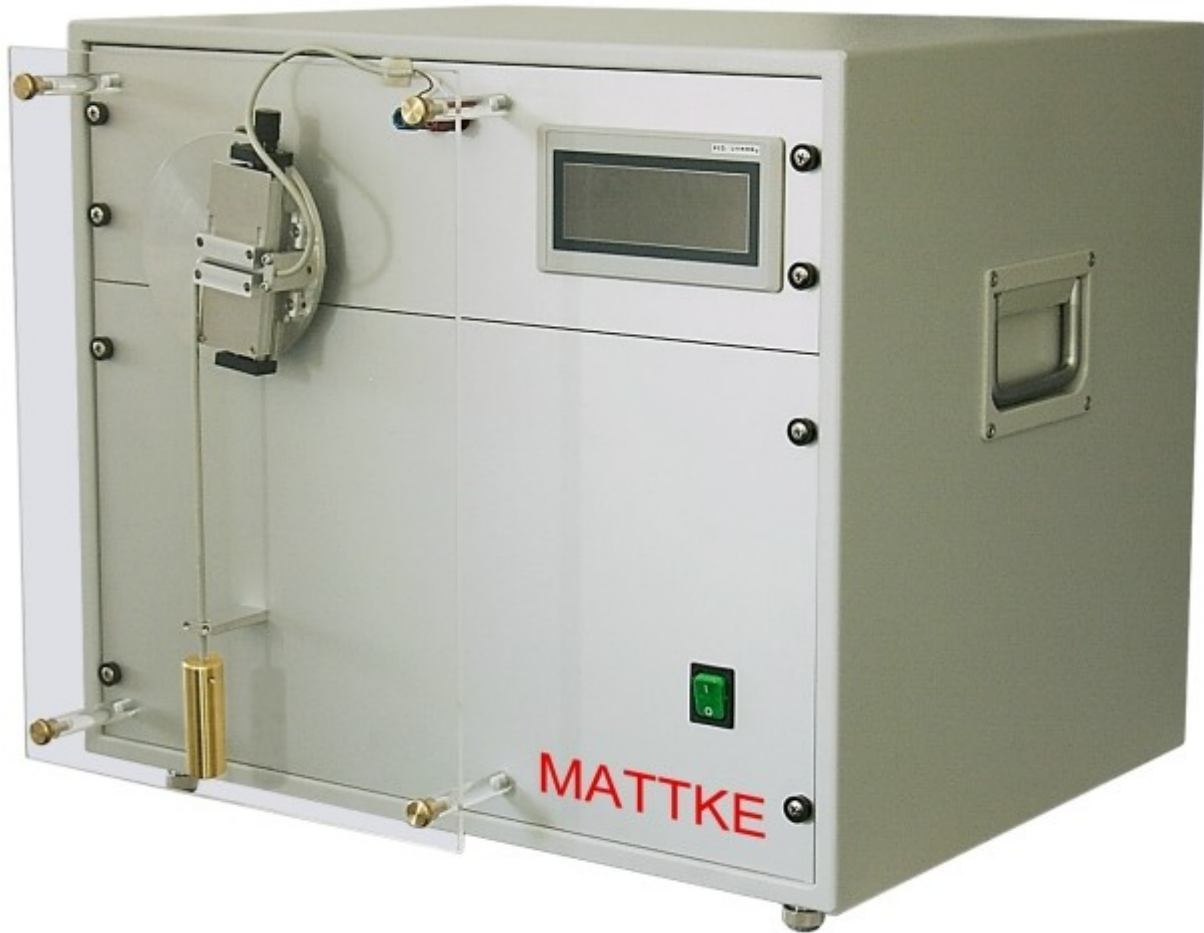
Single-axis Cable bend-test machine
