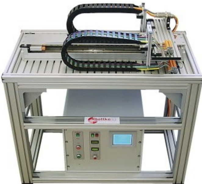
Cable test machine for 5 cables
